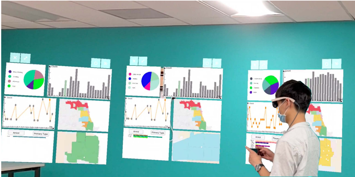
Figure 1: A user explores the Chicago crime dataset with SPARVIS, a cross-device system that combines a smartphone as an adaptive controller and AR glasses as a display. In the system, the user opens up three windows to compare crimes in different regions of Chicago at the same time. The user holds his smartphone horizontally so it is on trackpad mode and he can interact with visual elements within the selected window.
