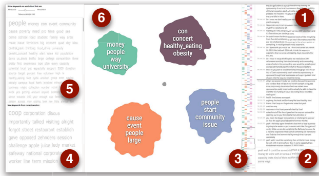
Figure 3: Iteration 1 of the interface features views seen in the final interface (Fig. 1) such as the transcript (1), real-time transcription (2), and word clouds of current (4) and previous (5) meetings. The main differences are a topics view (6) with relevant keywords overlaid on each topic “blob”, and a heatmap (3) showing topic probability distributions for each transcript line. New utterances merge into each topic blob, or an “unknown” topic blob in the center.
